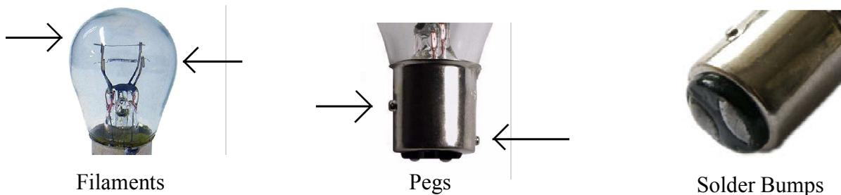
If you look at a typical dual purpose (dual circuit) tail lamp you will notice two offset pegs on the base of the lamp itself. These are for polarizing the base so it will connect to the socket connector only one way (unless you really force the lamp into the socket the wrong way, then you will have the Parking & Brake lights reversed). With all else being normal, the pegs make sure that the Brake and Parking elements are connected to the correct vehicle circuitry in the socket.
