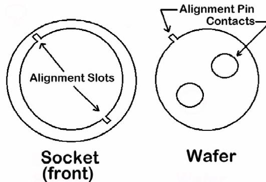
To test whether the wafer has slipped back into its socket shell backwards (or 180 degrees out of sync), take a dual filament incandescent lamp, plug it into the socket, taking note that the wafer alignment peg is fully seated in the slot in the socket.
