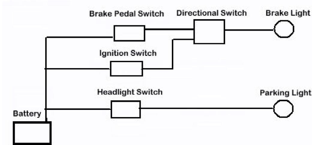
Power is routed to the Brake Light system from the Battery through the Brake Pedal Switch, through the Directional Signal Switch and on to the dual purpose tail lamps. Power for your Parking Light system is routed from the Battery, through the dash mounted Headlight Switch to the dual purpose tail lamps. The Directional Light system power comes from the Battery, through the Ignition Switch, through your Directional Signal Switch to your dual purpose tail lamps.
