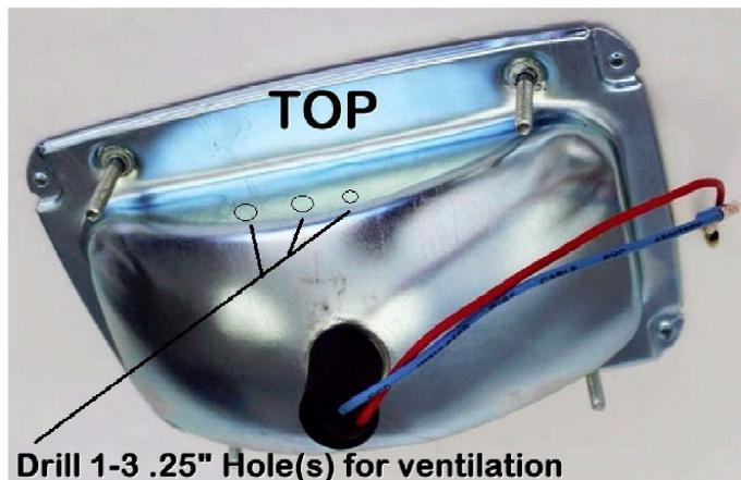
For a few installations, the design of the 64-66 tail light tub does not provide for sufficient cooling of the LED circuitry in our Sequential Brake Light System, and results in premature failure of the onboard LEDs.
