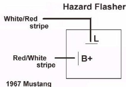
For most vintage Mustangs the flasher is located behind the dash board above the instrument cluster. Not the easiest place to have to locate something that needs to be relatively often. On some 1965 Mustangs, the Flasher is located in a clip behind the fresh air vent on the driver's side. Also '67-'68 Mustangs may have an extra flasher for 4-way (Emergency) Directionals. Make sure you are replacing the correct one - they look identical.
